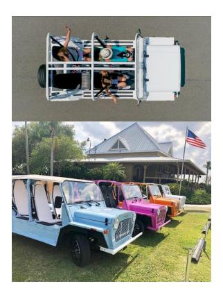
Suspension (Front): MacPherson Independent Suspension (Back): Lengthways **Trailing Arm** Brakes: Hydraulic Four Wheel Front Disc/Rear Drum Parking Brake: Hand Lever Body (Front, Rear & Finish): Painted Tires: 175/60R14 DOT Rated Wheelbase: 89" Inches **Overall Height:** 61" Inches Overall Length: 131" Inches Overall Width: 65" Inches Curb Weight: 2,200 Pounds **Ground Clearance** (Differential): 7.5" Inches
